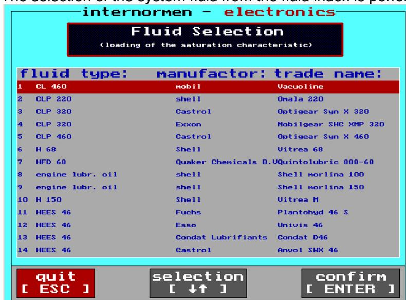
Select the fluid using the [ ↓↑ ] – keys (selection is highlighted red) and confirm with [ENTER].
